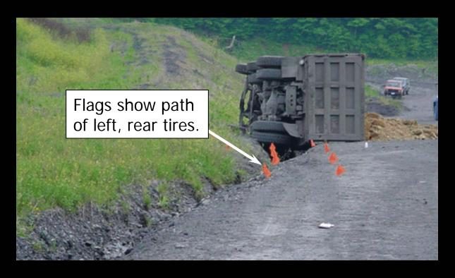
The victim, a 52-year old heavy equipment operator with 26 years of mining experience, was operating a refuse truck while descending a grade from the crest of an impounding structure. He lost control of the truck during the descent, causing the truck to leave the roadway, travel across a ditch, and overturn. The driver was found along the ditch, approximately 60 feet uphill from the truck.
