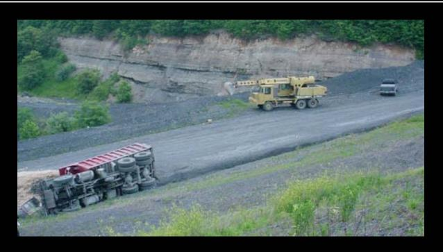
Prior to the accident, the brakes of the truck were not tested to determine if they were sufficient to stop and hold the loaded truck on the grade where it was being used. Procedures were not in place to test the brake system. A physical examination of the brake systems and components of the truck had not been made since the truck was leased for use at this site.
