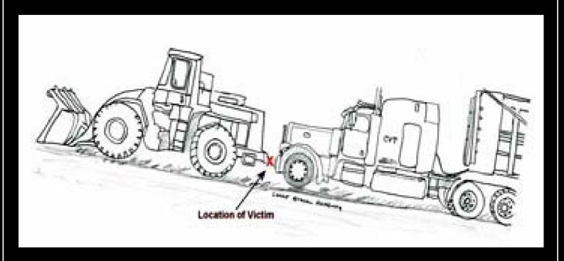
On November 9, 2004, a 57-year old mine owner with 30 years of mining experience was fatally injured while helping to install a steel pull rope (tow rope) from the rear of a Caterpillar 980C front-end loader to the front pull hook of a stalled Peterbilt tractor-trailer coal truck. The front end loader inadvertently rolled backwards down the inclined roadway towards the tractor-trailer, pinning the victim between the two pieces of equipment.
