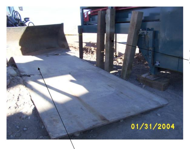
Timbers used to support plate so it Would not hit the plant.
