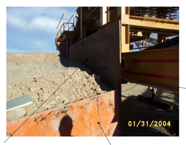
Side plate (wing) welded to back plate.
