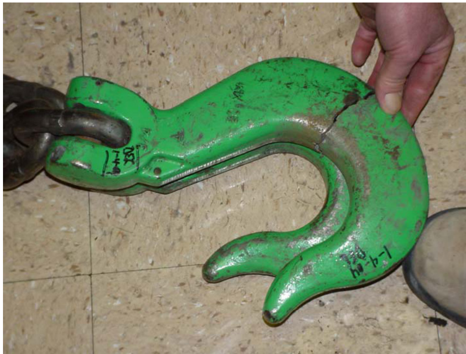
BROKEN HOOK LAYING ON TOP OF OTHER HOOK FROM 2-LEGGED CHAIN SLING
