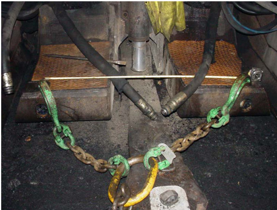
RE-ENACTMENT OF SLING ATTACHED TO TOES OF NO. 49 SHIELD VICTIM WAS LOCATED ON THE RIGHT SIDE SHIELD TOE
