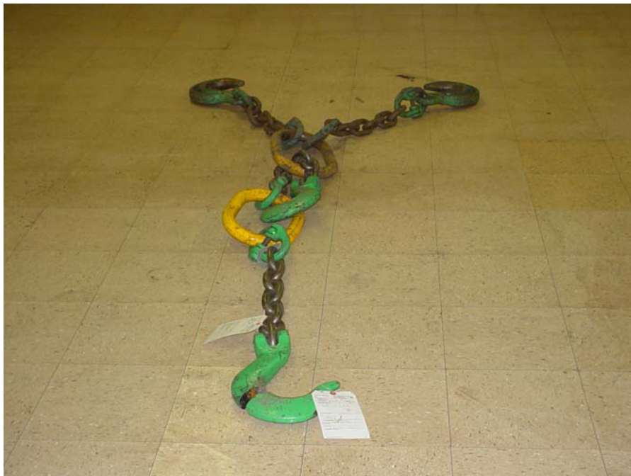
THE TWO 2-LEGGED CHAIN SLINGS AS RIGGED DURING ACCIDENT THE BROKEN HOOK IS IN FOREGROUND WITH WHITE TAG ATTACHED
