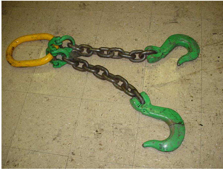
2-LEGGED CHAIN SLING WITH BROKEN HOOK
