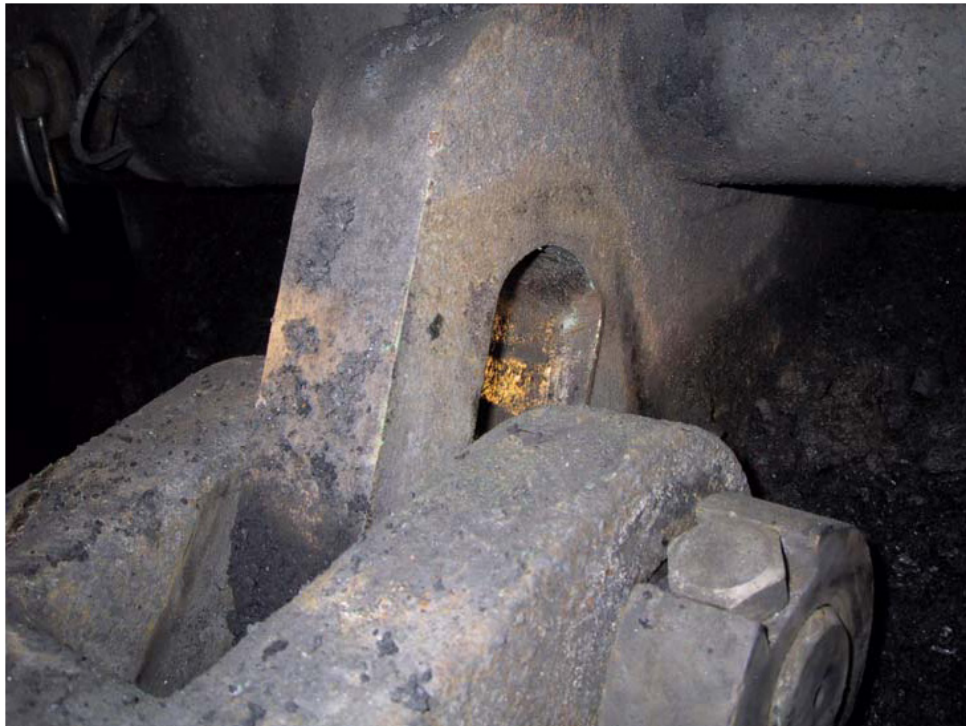
SLOTTED HOLE ON FACE CONVEYOR WHERE HOOK WAS INSERTED
