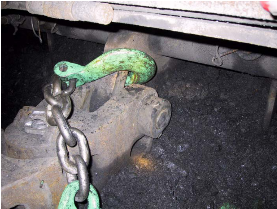
RE-ENACTMENT OF HOOK INSERTED INTO SLOTTED HOLE ON FACE CONVEYOR
