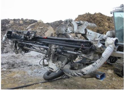
Drill mast in lowered horizontal position for manually placing steels in the magazine.
