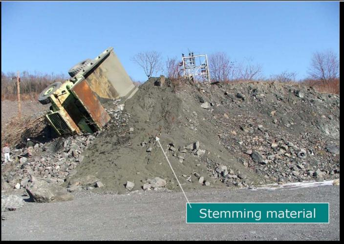
A Caterpillar haul truck driver, arrived at the rock refuse dump and saw the Euclid R-85 haul truck on its side. The victim, who received fatal injuries, was inside the operator's cab. The truck's engine was still running and the rear tires were spinning. As rescue operators were attempting to enter the truck, the engine stopped.
