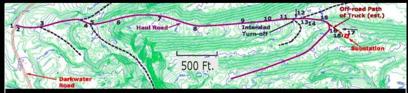
The pit was accessed via an unpaved haul road. This haul road was approximately 4,000 feet long and ranged in width from 50 to 75 feet. The haul road surface was reasonably smooth and clear of snow. Although portions of the haul road were frozen, they were not icy. Left side tire marks were visible on a rock refuse bank approximately 600 feet from the accident scene. This area of the haul road had a variable grade of 9.6 to 14 percent.
