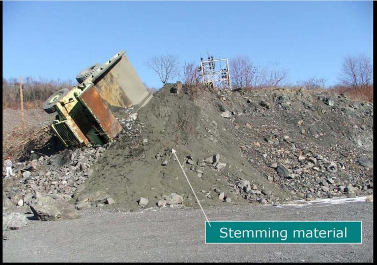
The truck involved in the accident was a 1975 Euclid R-85 haul truck. The net vehicle weight (light weight) of the truck was 117,100 pounds. The estimated weight of the load at the time of the accident was 170,000 pounds (85 tons). The gross vehicle weight of the truck was 287,100 pounds.
