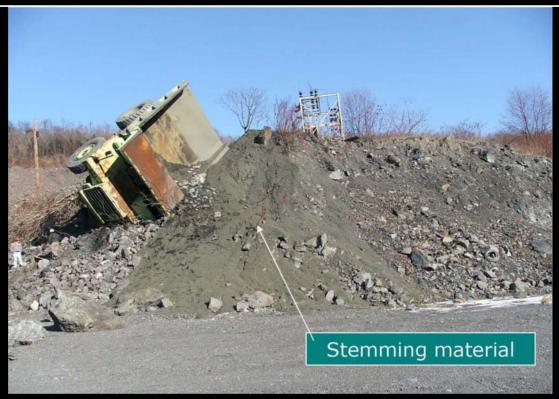
The foreman requested the mechanics to start a haul truck to transport stemming material. The mechanics started a Euclid R-85 haul truck, Company No. 671. This truck was used primarily to haul stemming material but had not been operated for four to six weeks.
