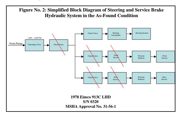
The effect of these defects did not allow the forklift to maintain pressure in either of the two service brake circuits once the engine was shut down.
