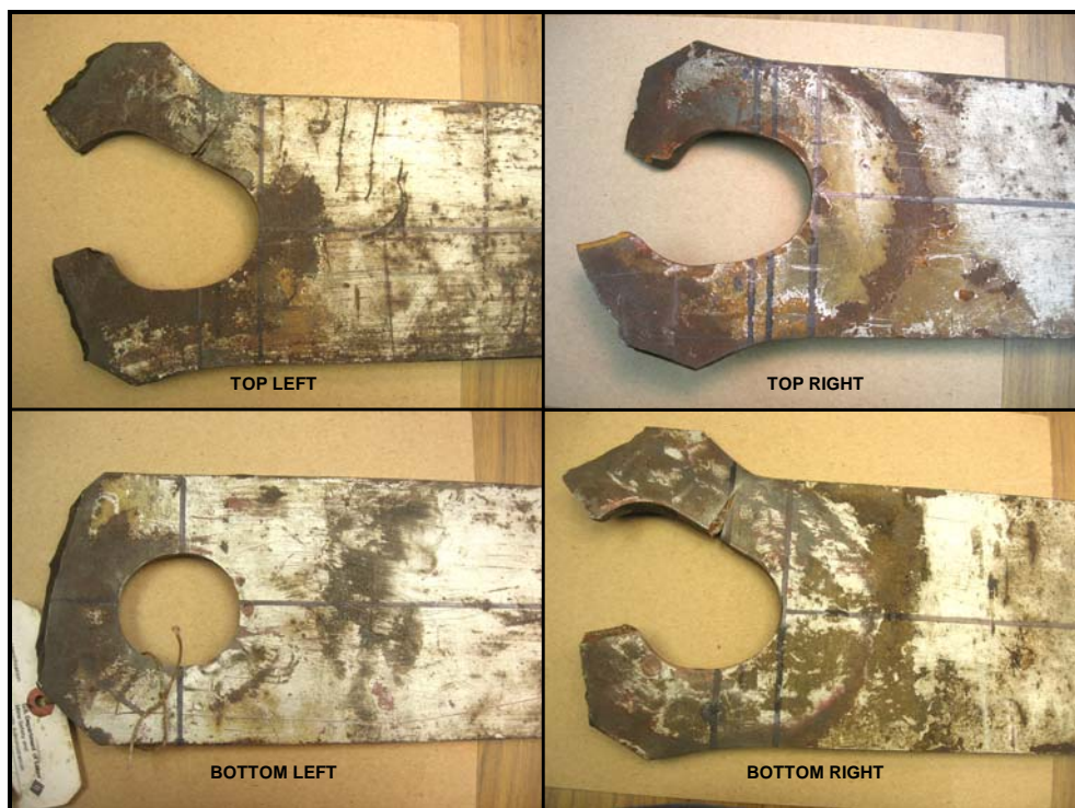
Photo 2 - Anchor arm conditions after pin connection failed.
