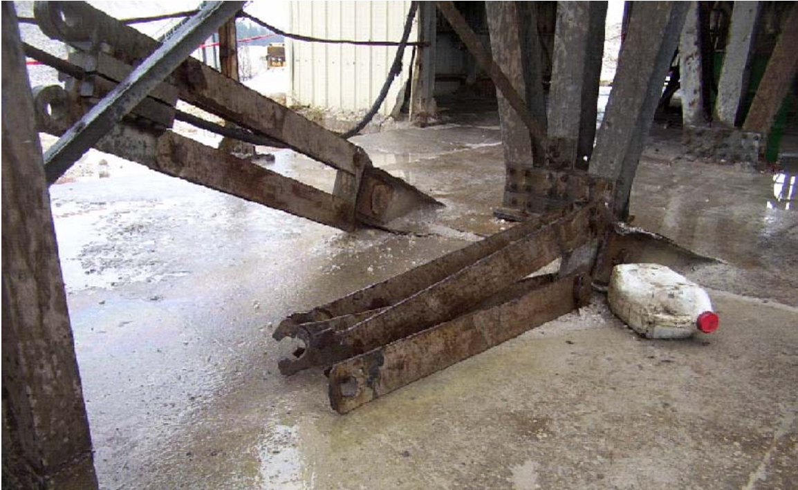
Photo 1 – Empty cable anchor arm assembly and failed load cable anchor arms.
