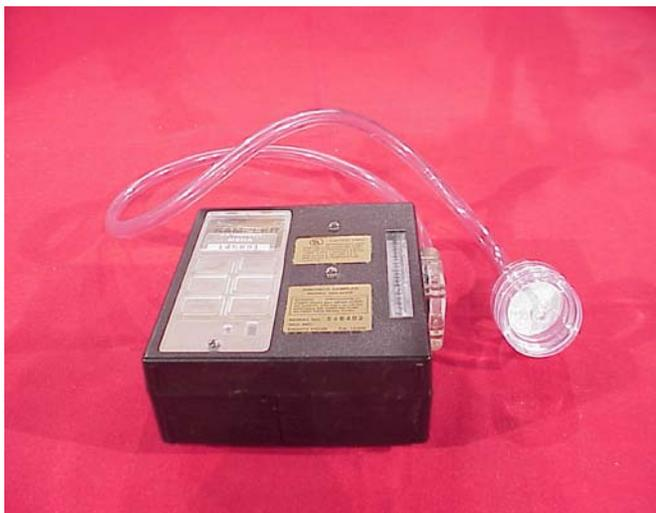
**Figure 7-2. Welding Fume Sampling Train**
