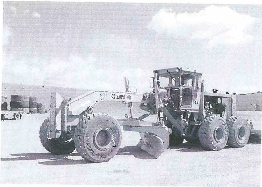
Figure A.13. Caterpillar 16G motor grader.
