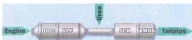
Fig. 1 Schematic representation of diesel engine after treatment technologies. DOC diesel oxidation catalyst, DPF diesel particulate filter, SCR selective catalytic reduction, AMOX ammonia oxidation catalyst. Published with permission from the Health Effects Institute
