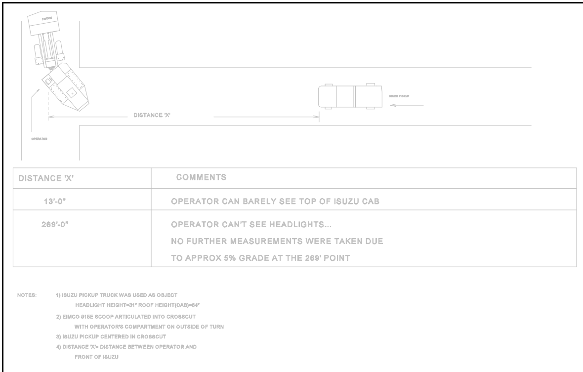
Figure 11 – IN MINE BLIND SPOT SURVEY – SCOOP ARTICULATED INTO CROSSCUT
