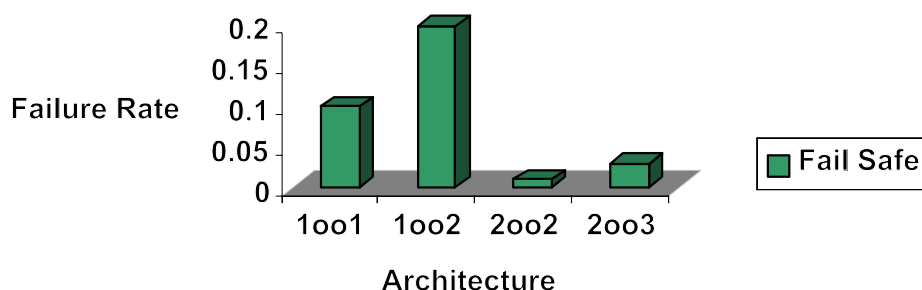
Figure 11.—Safe failure rates for various switch architectures.
