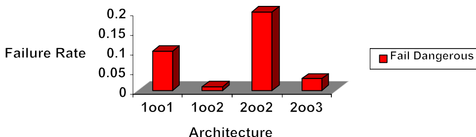
Figure 10.—Dangerous failure rates for various switch architectures.
