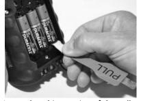
5. Insert the white section of the pull tab between the battery on the right and its contact inside the compartment. Hold the pull tab in place with one hand while using the other to replace the compartment cover.
