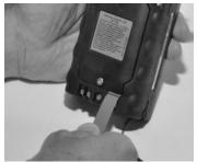
1. Remove the pull tab on the back of the instrument by pulling it straight out. Set the tab aside.
