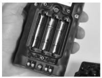
3. Ensure the instrument is powered off, loosen the captive screws, and then remove the cover. Remove and discard the alkaline batteries. Inspect the battery compartment. Replace it if there are signs of dust, water, corrosion, or discoloration.
