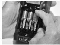
4. Insert three new batteries using the postive (top) and negative (bottom) orientation shown here.
