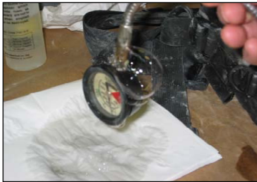
Figure 6a: Leak at chest gauge.on Apparatus #15
