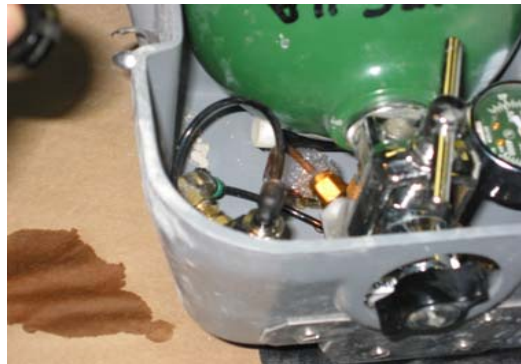
Figure 6c: Leak at T-connection on Apparatus #15
