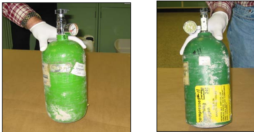
Figure 2: Cylinder BA253, with a non-standard gauge, next to cylinder WJ173, with standard gauge.
