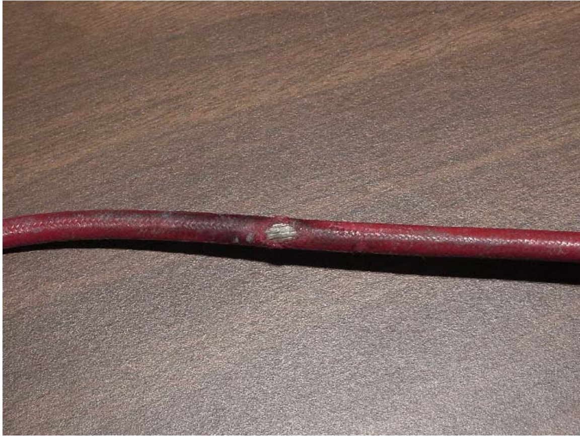
6. Damaged Area of C-Phase Power Cable
