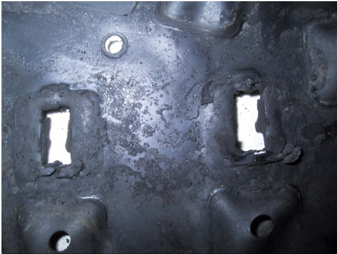
Figure 3. PE-1 Transmitter, Front Panel cover plate, gasket side view, detail, tram lever openings
