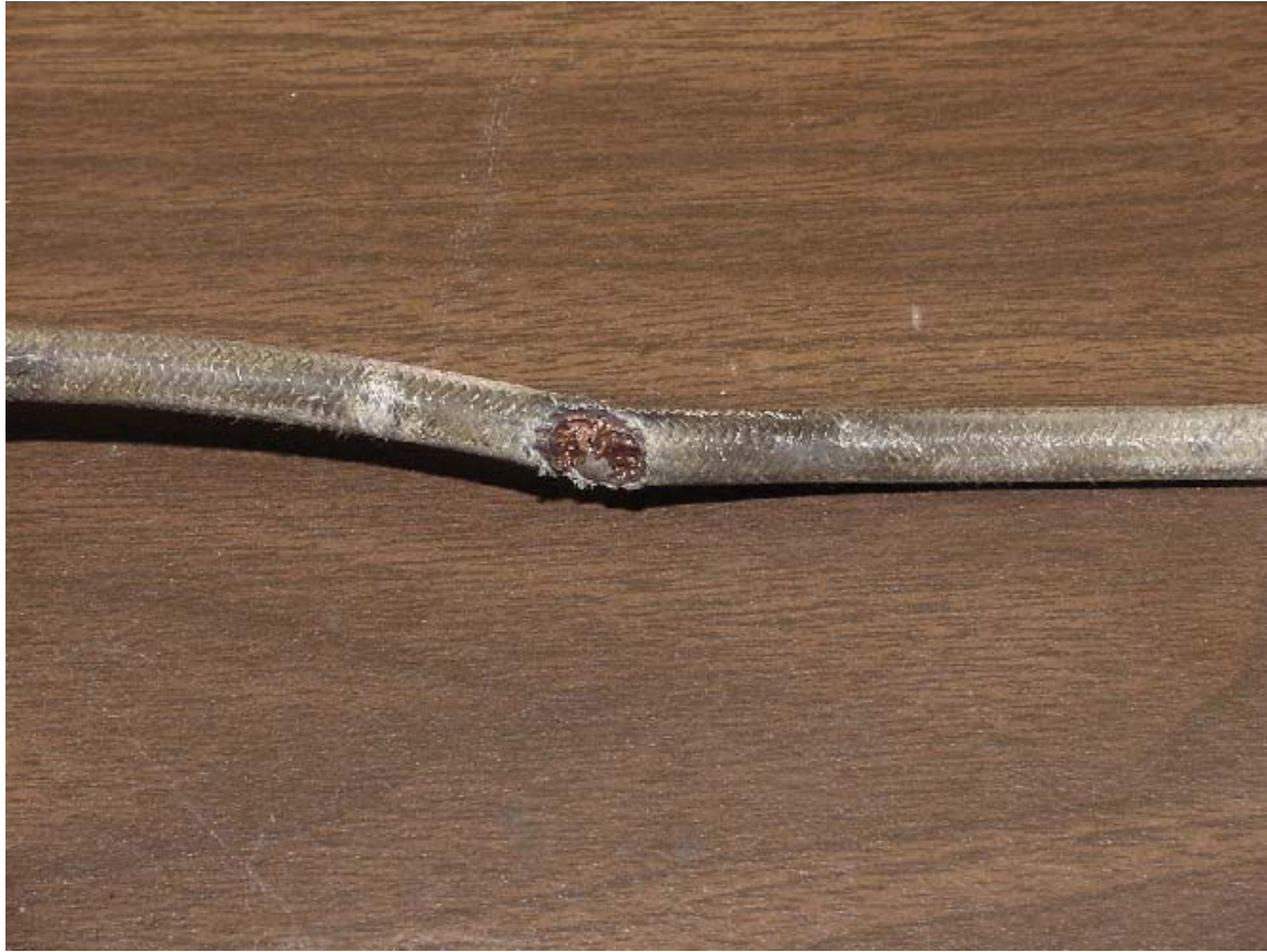
5. Damaged Area of B-Phase Power Cable
