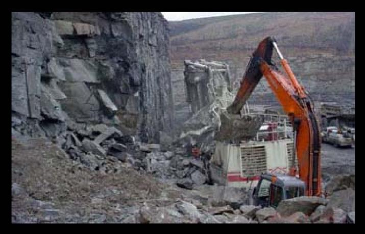
A 41-year old equipment operator with seven months of mining experience was fatally injured while operating an excavator near the highwall, loading spoil into trucks. The excavator was positioned with the cab on the highwall side. The highwall collapsed causing rocks to cover the operator's cab.
