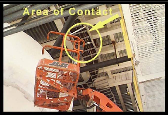
At 8:05 a.m. on Friday, July 7, 2006, a 35-year old Millwright was fatally injured while operating a JLG Lift, Model E300A. The accident occurred while the victim was repositioning the platform of the lift beneath the second floor of the preparation plant. The victim was caught between a metal cable tray and the handrail over the platform control panel resulting in fatal injuries.
