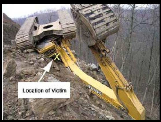
At approximately 4:00 p.m. on March 12, 2007 a 47-year old foreman/excavator operator with 29 years mining experience received fatal injuries when the track-mounted excavator which he had been operating overturned from an elevated mine bench. The victim had been loading and moving shot rock overburden while positioned on the narrow
