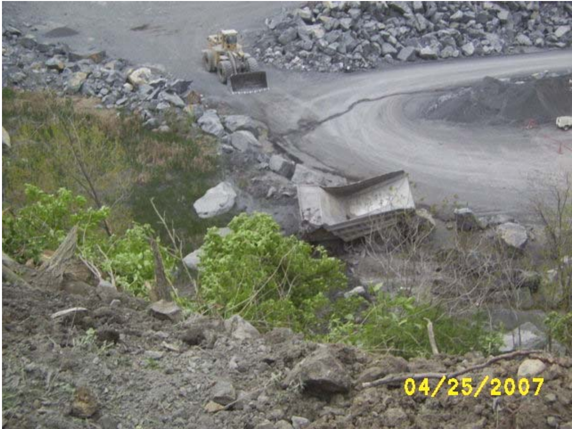
View of haul truck on the 740 Level where it landed after rolling from roadway above.
