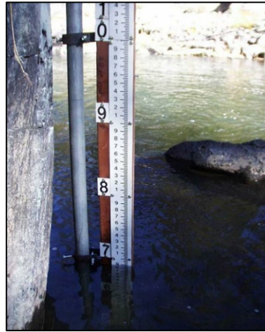
Photo 32. Staff gauge showing depth.
