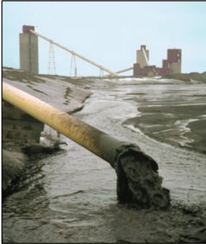
Photo 3. Delivery of fine refuse to a coal impoundment.
