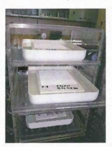
7. Carefully pour 800 ml (do not overfill) of distilled water into each water tray. The 800 ml of added water should reach nearly to the top of the sample trays.
