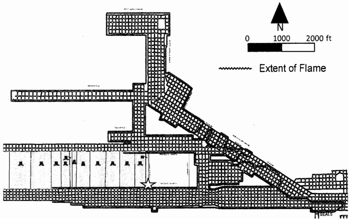
**Figure 12** — Extent of the flame zone of the Upper Big Branch Mine explosion. The star indicates the origin of the explosion on the tailgate side of the longwall face. Modified after Page et al. (2011).
