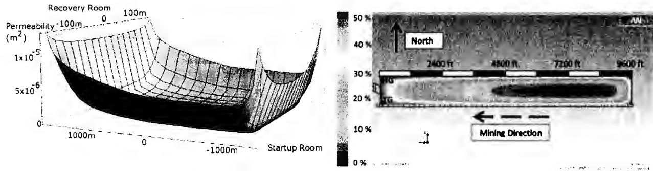
**Figure 13** — Longwall gob permeability (left) and resulting porosity distribution (right), from Worrall et al. (2012).
