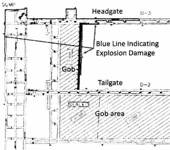
**Figure 10** — Map of the Willow Creek Mine 2000 explosion after McKinney et al., 2001, no scale indicated).
