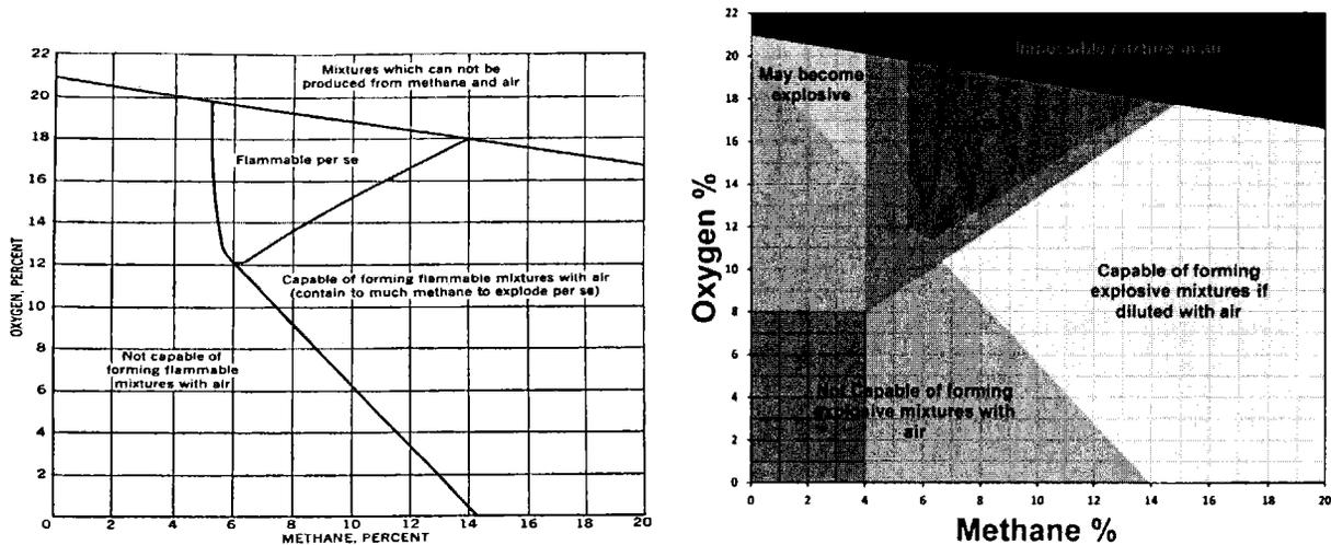
**Figure 3** — Methane explosibility diagram by Coward and Jones (1952), along with the color coding scheme used to characterize EGZs. The orange area surrounding the red, explosive zone is an arbitrary buffer zone indicating a gas mixture close to explosive. The blue area may become explosive if methane is added. The yellow area may become explosive if the mixture is diluted with oxygen. Green areas are inert.
