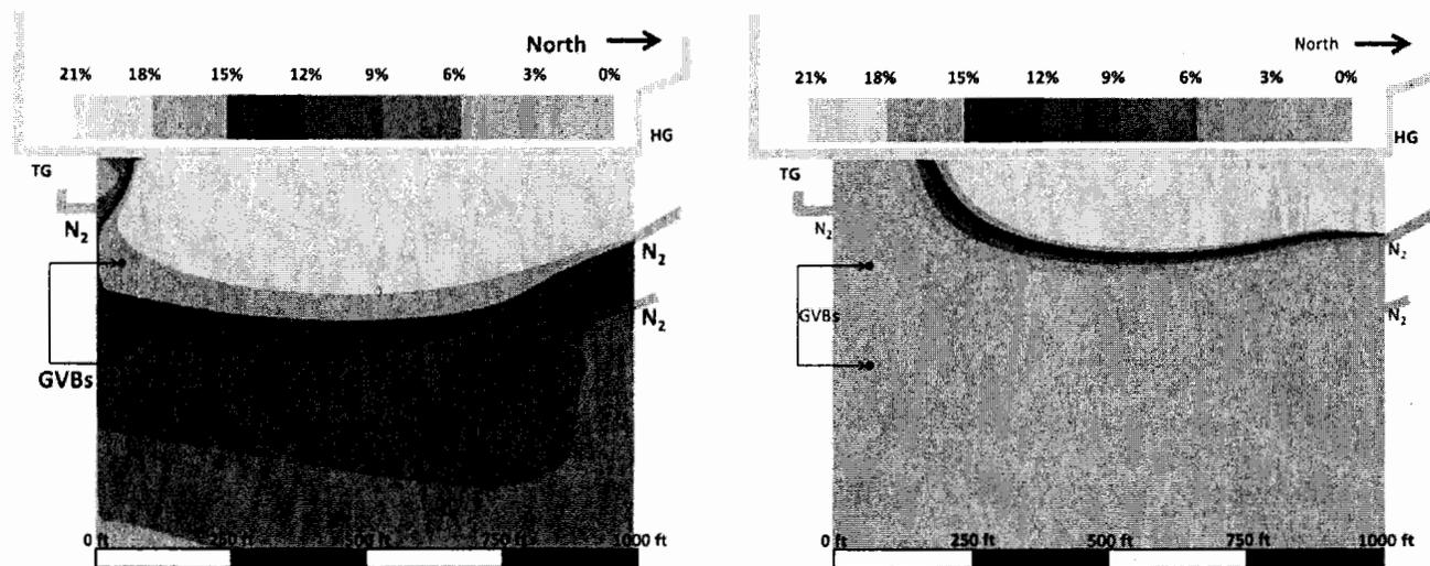
**Figure 16** — Reduction of oxygen penetration into the gob by increasing nitrogen injection quantities from 0.1 (left) to 0.4 m<sup>3</sup>/s (right) (200-800 cfm) on both headgate and tailgate sides (Marts et al., 2013).
