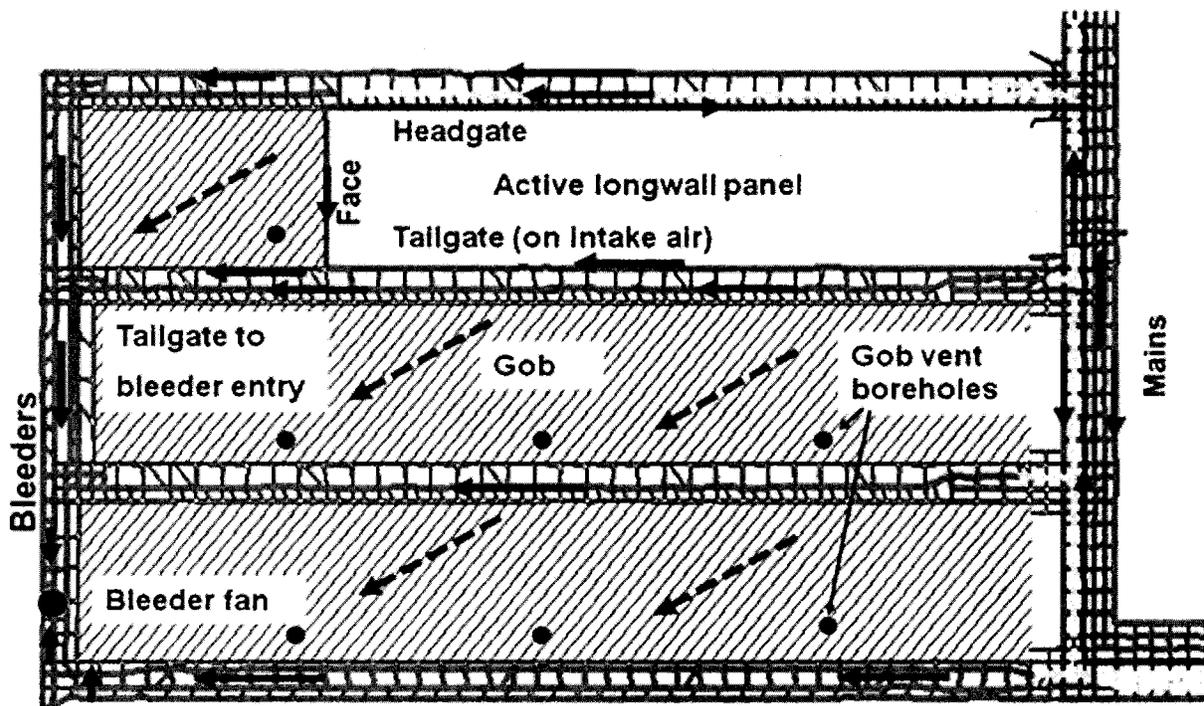
**Figure 2** — Typical longwall mine bleeder ventilation scheme. Arrows indicate direction of air flow. Colors indicate fresh air (intake): green; track: yellow; belt: blue; return or bleeder air: red. Black dashed arrows indicate general air flow tendencies in the gob. After Brune et al. (1999); not to scale.
