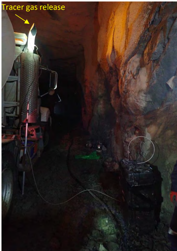
Figure 1: Tracer gas release into the Agi truck exhaust.
