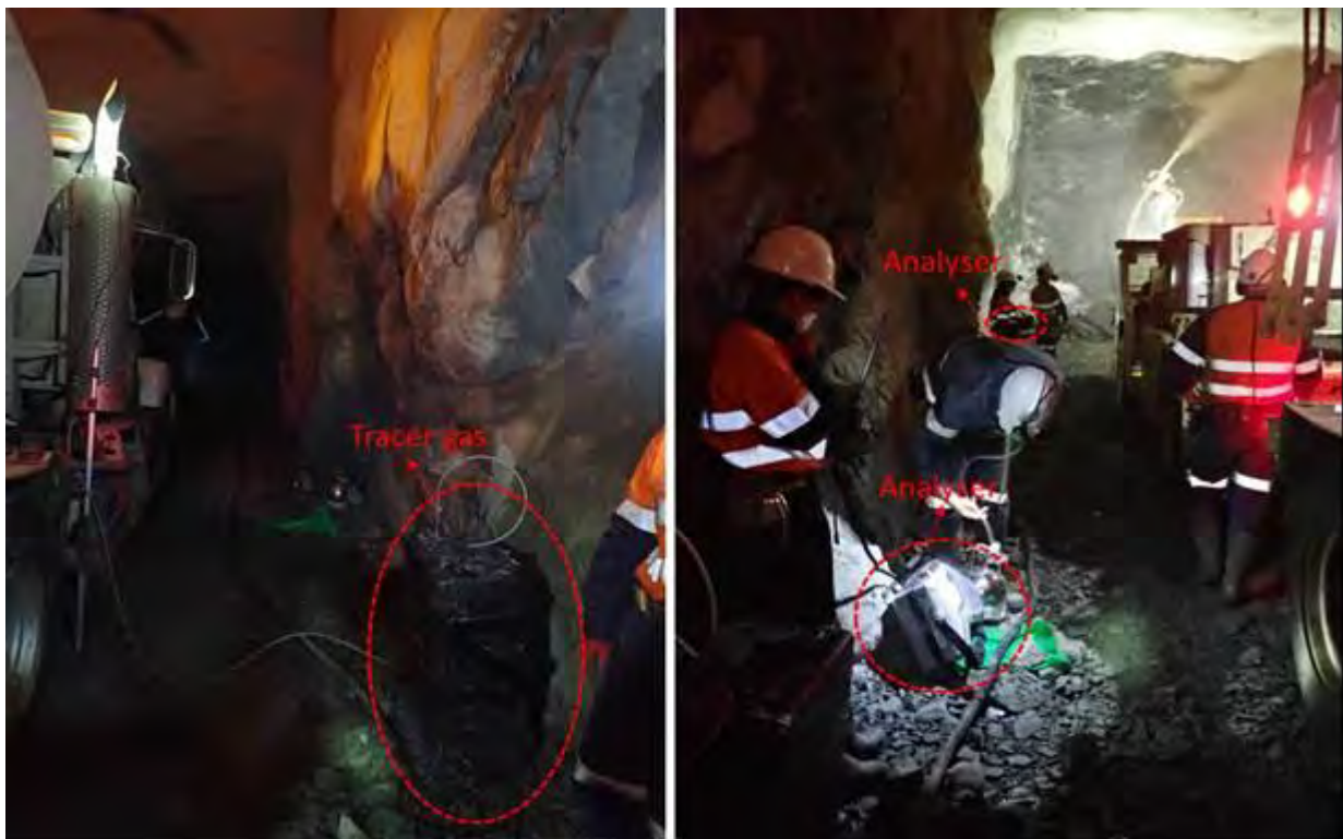
Figure 9: Tracer gas study during the Hydro-scaling and Shotcreting activities.
