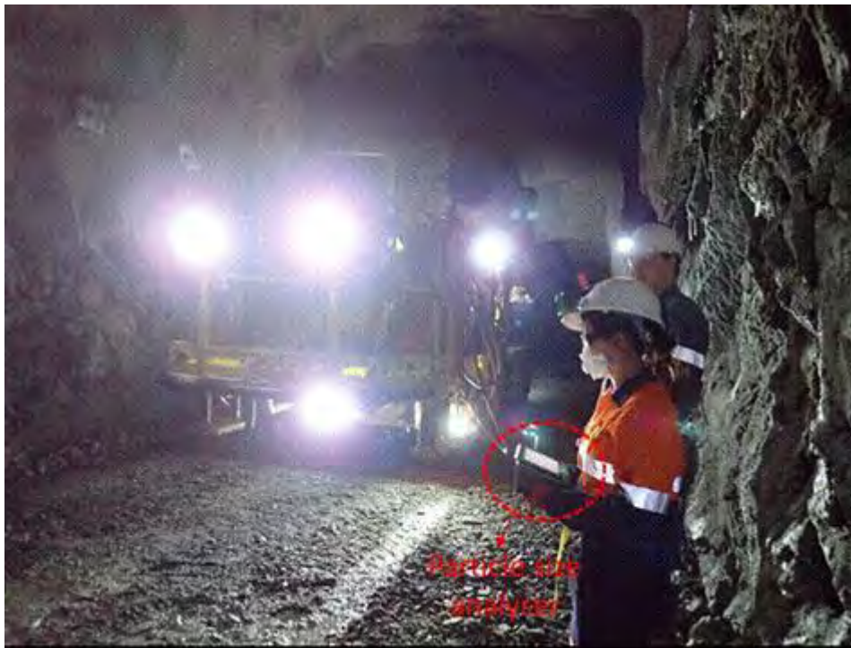
Figure 5: Particle size monitoring during the Charging activity.
