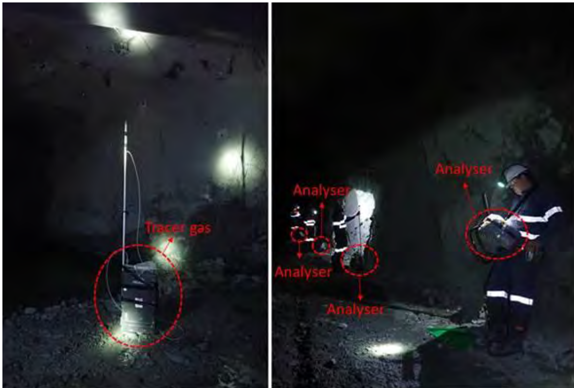
Figure 15: Tracer gas study during the Traverse exercise.
