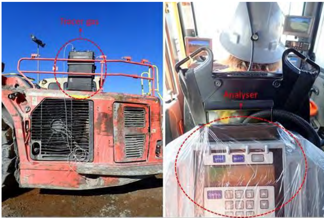
Figure 12: Tracer gas study during the Truck activity.
