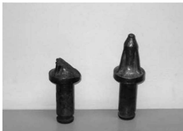
FIGURE 1. Comparison of worn miner bit (left) to a new bit (right). Reproduced with permission from Pollock et al. 27
