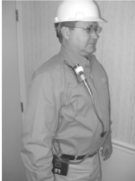
FIGURE 3-1—RESPIRABLE DUST SAMPLING SETUP
