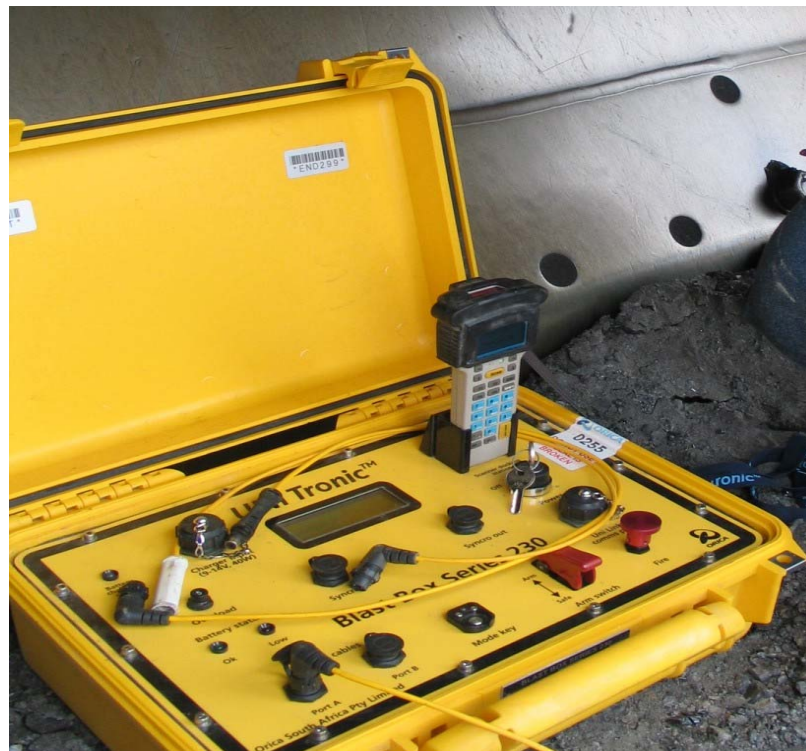
Figure 8 -- Orica UNI Tronic™ Blast Box with the Scanner inserted to download electronic detonator information
