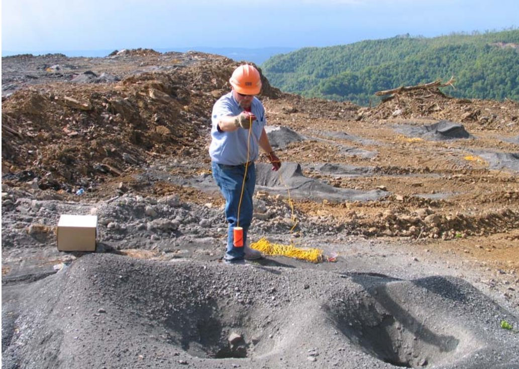
Figure 13 – Priming a blasthole with a booster prior to loading with ANFO-emulsion blasting agent
