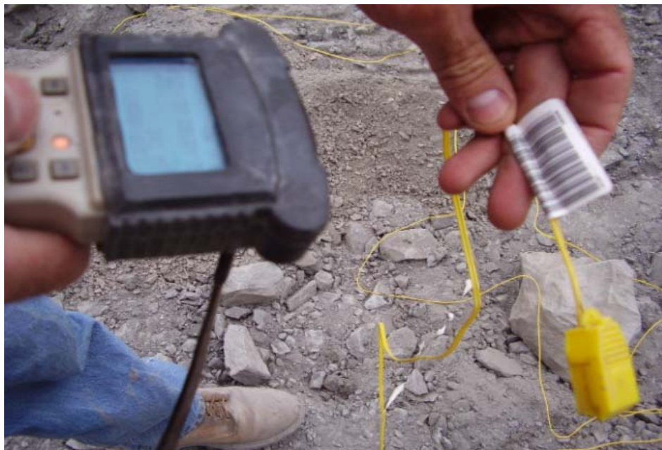
Figure 10 – Orica UNI Tronic™ Scanner used to read an electronic detonator (Unitronic™ 500) bar code ID
