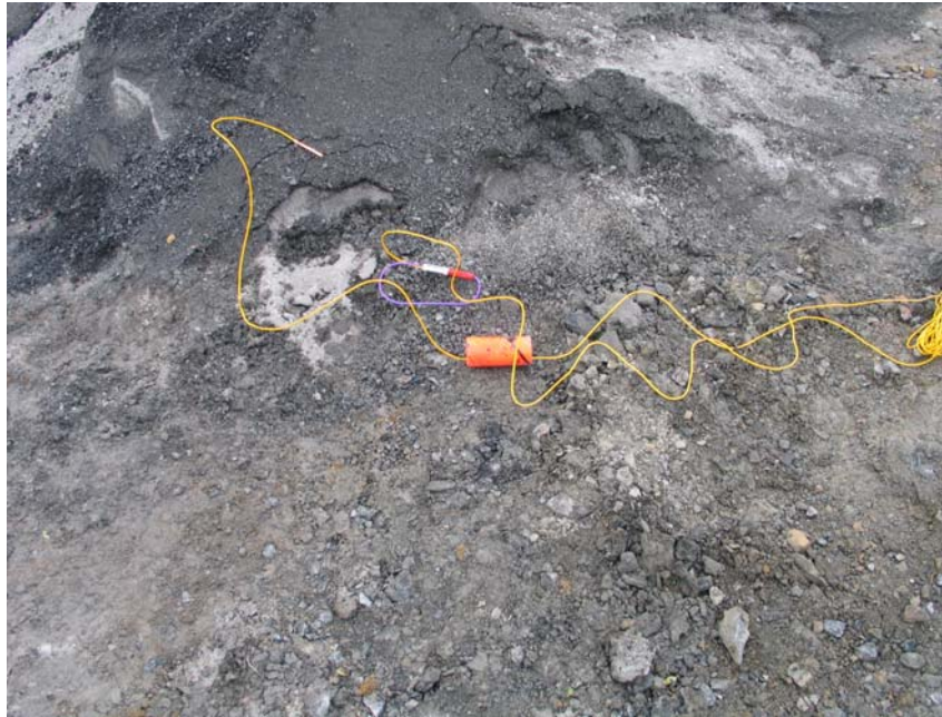
Figure 5 – Orica UNI Tronic™ 335 electronic detonator and booster
