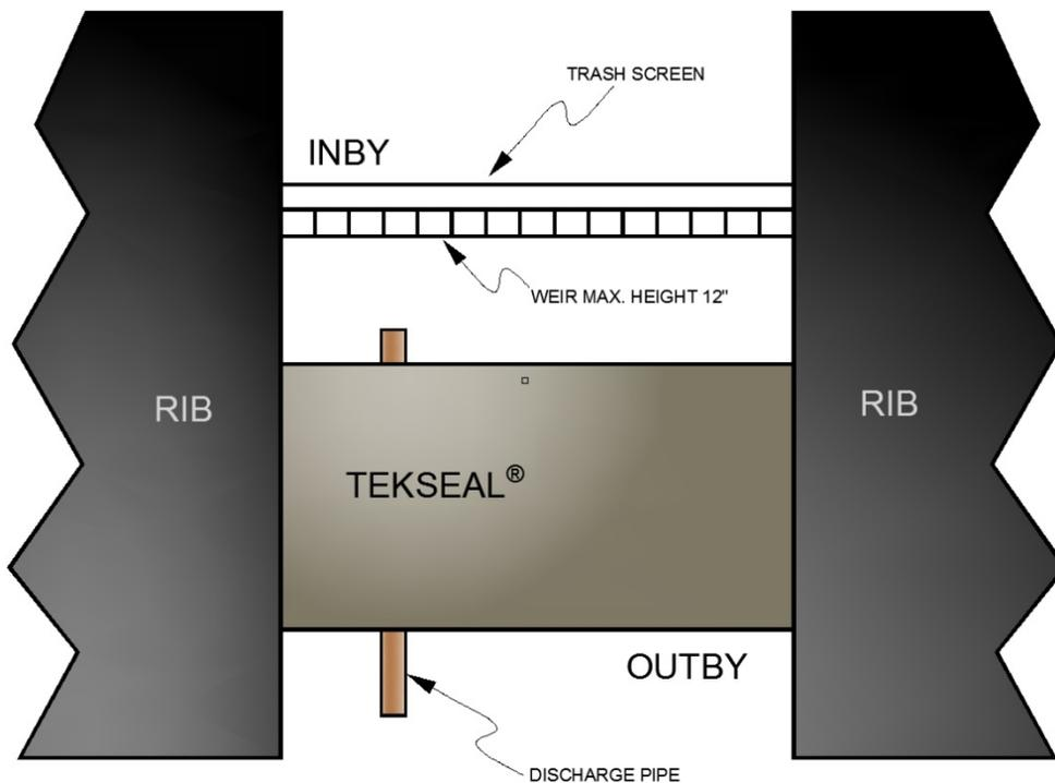
If a new seal is placed on the outby side of an existing seal equipped with a water drainage system, the existing U-trap must be removed, the existing valve must be removed or placed in a fully-open position, and the drainage pipes must be extended through the new seal with a new valve
