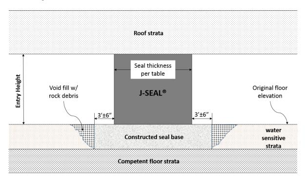
While constructing the base, the excavated cavity can be filled entirely with high strength grout, or similar material. Normal formwork can also be used for construction of the base. The formwork can remain in place or be removed once the base has achieved the minimum UCS per the sampling procedure. The excavated area can be backfilled with dirt and/or rock debris to the approximate original floor horizon.
