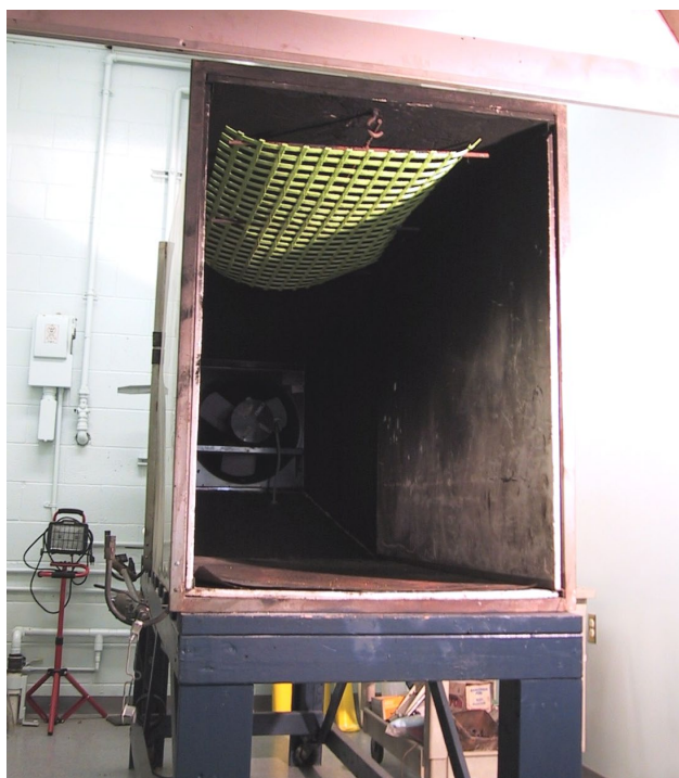
Photo No. 4: Roof-Rib Grid Material – Horizontal Flame Test
