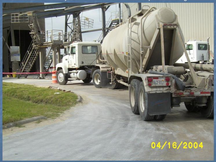
This picture illustrates the fold down cage provided for the truck drivers to protect them from falling while accessing the hatch at the top of the trailers. The victim fell between the rails and the trailer to the ground.
