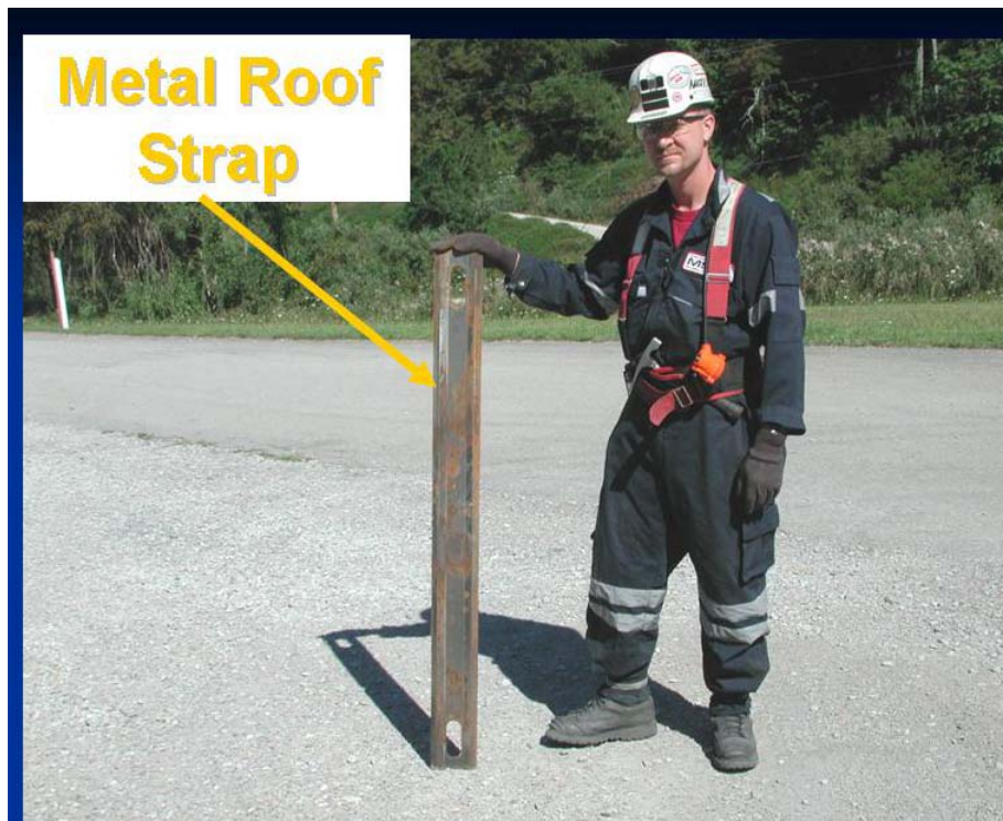
FIGURE 1. MSHA EMPLOYEE HOLDING METAL ROOF STRAP
