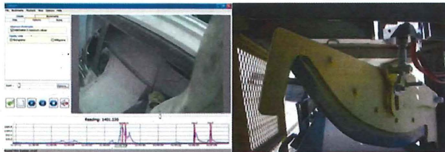
Figure 3 - Left side shows screenshot of EVADE software of miner performing manual deployment of scraper device with high peak in dust exposure shown in the bottom of the screen; right side shows photo of new pneumatic system to eliminate worker performing the task.
