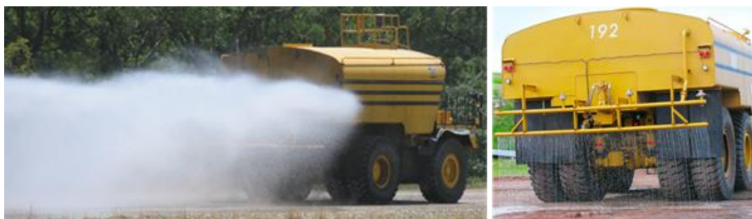
Figure 11.7. Water trucks wetting down haul roads. The left photo shows a water truck with rear-mounted water sprays and the right photo shows a haul truck with a water distribution manifold.
