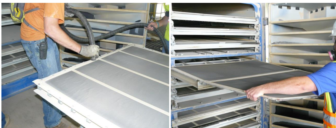
Figure 9.14. Photos of a worker vacuuming a regular screen and a worker removing a new segmented panel screen. The left photo shows the worker vacuuming exterior cloth fabric material around the screening clips and screen housing bracket. The right photo shows a “segmented panel” screen design made up of three different panels that clip together.
