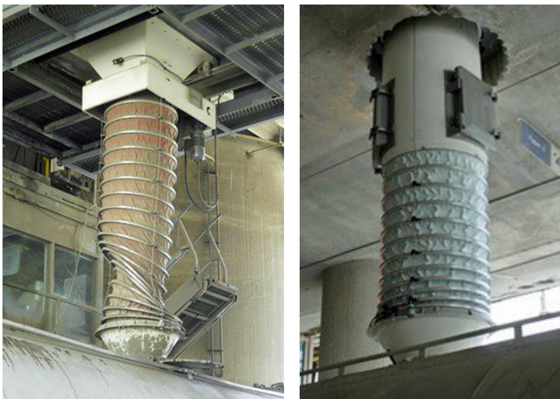
Figure 8.6. Photos of loading spouts under different levels of negative pressure. The photo on the left shows excessive exhaust flow collapsing the spout while the photo on the right shows an acceptable level of exhaust pulling the outer shroud fabric but not collapsing the spout.
