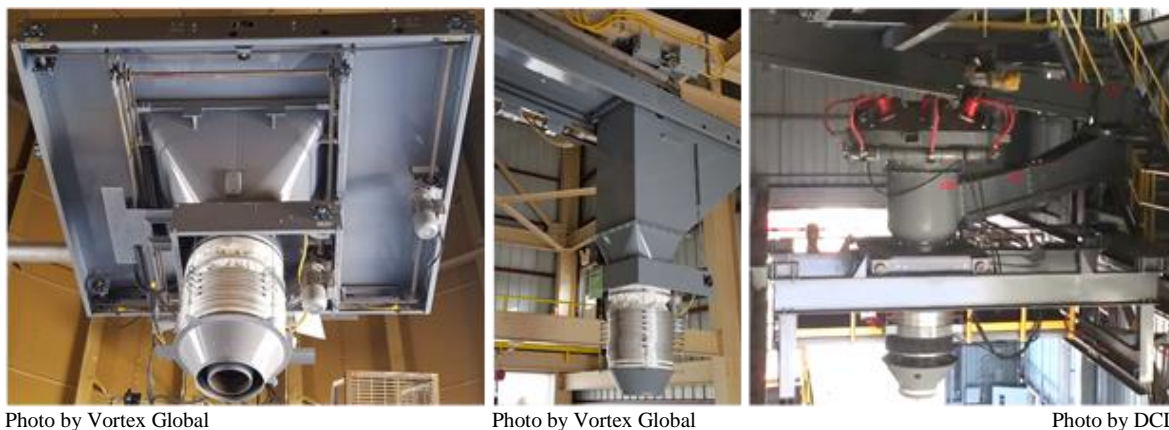
Figure 8.3. Three types of loading spout positioners. The left photo shows a dual-axis positioner, the center shows a rotating positioner, and the right shows an articulating arm positioner.
