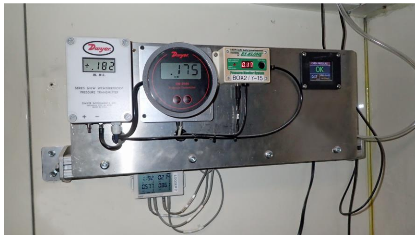
Figure 10.16. Comparison test of three pressure monitors at a crusher booth at an underground mine compared to a certified pressure reference instrument. The Dwyer gauge is on the far left.
