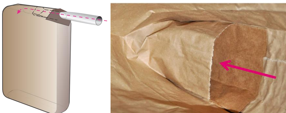
Figure 7.2. Fill nozzle and bag valve. The left illustration shows a typical bag valve. The right photo shows an interior view of a bag valve. The fill nozzle enters through the bag valve and delivers product into the bag.
