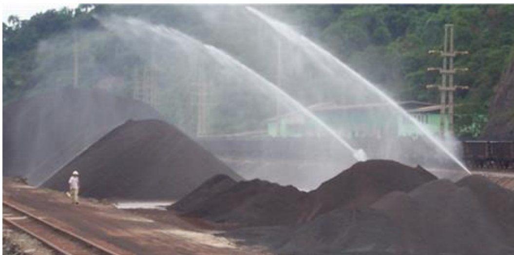
Figure 11.13. Long-throw sprinklers wetting stored material [from Rain Bird Corporation 2009].
