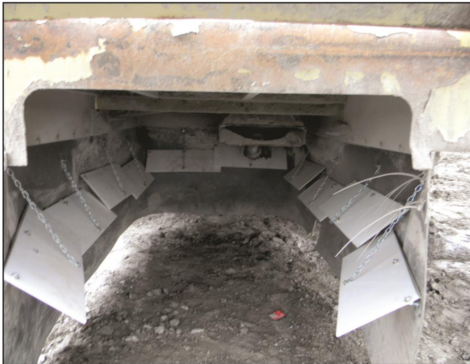
Figure 4.14. Air-blocking shelf with modifications incorporated into installation. This shelf was installed in short sections in an attempt to prevent potential damage that could occur during tramming with the drill mast up. Note that each of the sections overlap, eliminating any gaps in the shelf perimeter.
