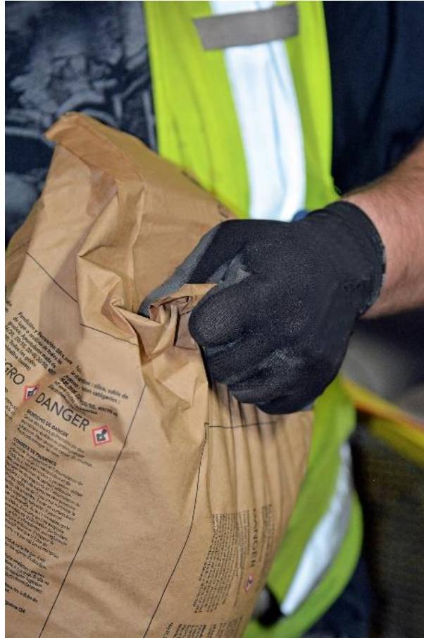
Figure 9.22. Worker squeezing the bag valve closed with his hand as he removes the bag from the fill nozzle, significantly reducing his dust exposure.
