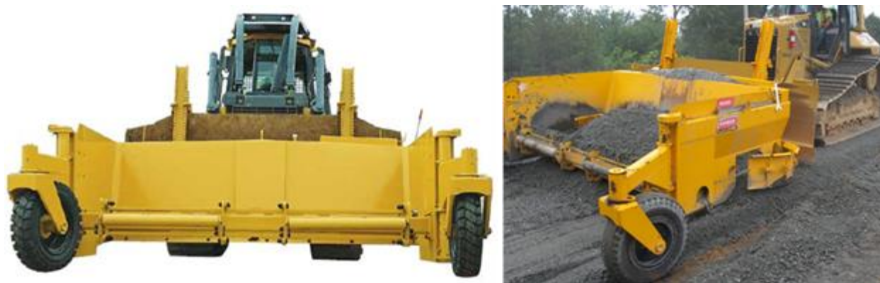
Figure 11.6. Photos of a spreader box used to spread the material for the base of a haul road. The left photo shows an aggregate spreader mounted onto a bulldozer blade and the right photo shows base material being spread onto a roadway.
