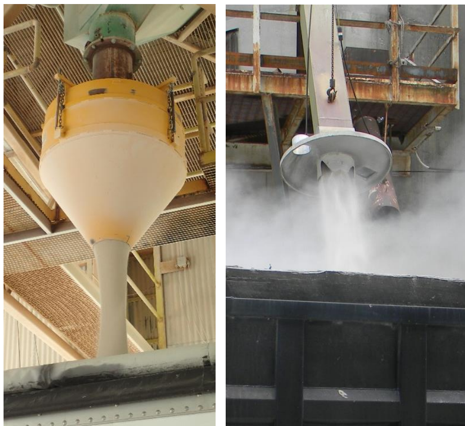
Figure 8.8. Demonstration of how a conical-shaped hopper installed at the product discharge point can minimize dust liberation during bulk loading. The left photo shows the Dust Suppression Hopper discharging a consolidated product stream versus an unconsolidated stream from a rigid spout in the right photo.
