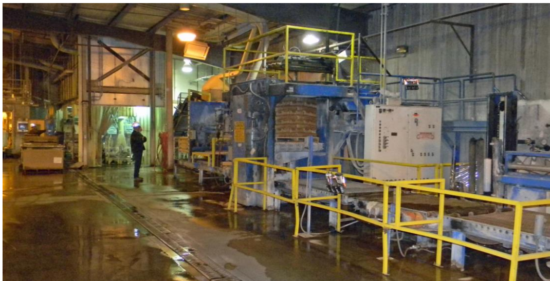
Figure 7.19. A typical high-level automated bag palletizing system. The top illustration shows an overhead view of the overall design. The bottom photo shows an automated high-level palletizing process in use.
