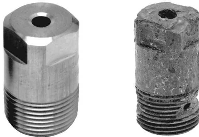
Figure 3.26. Temperature damage—new versus used [adapted from SSCO 2013].
