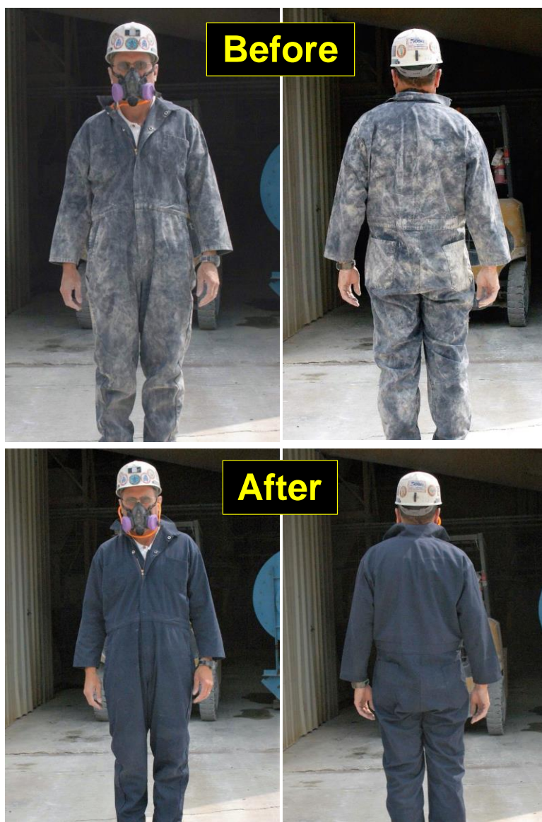
Figure 9.4. Test subject wearing polyester/cotton blend coveralls before and after using the clothes cleaning booth.
