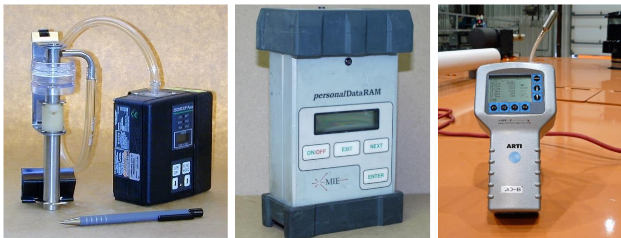
Figure 10.19. Three types of sampling instruments used for determining filtration and pressurization system effectiveness. The left photo shows a personal gravimetric sampler, the center photo shows a nephelometer light-scattering instrument, and the right photo shows a handheld optical particle counter.
