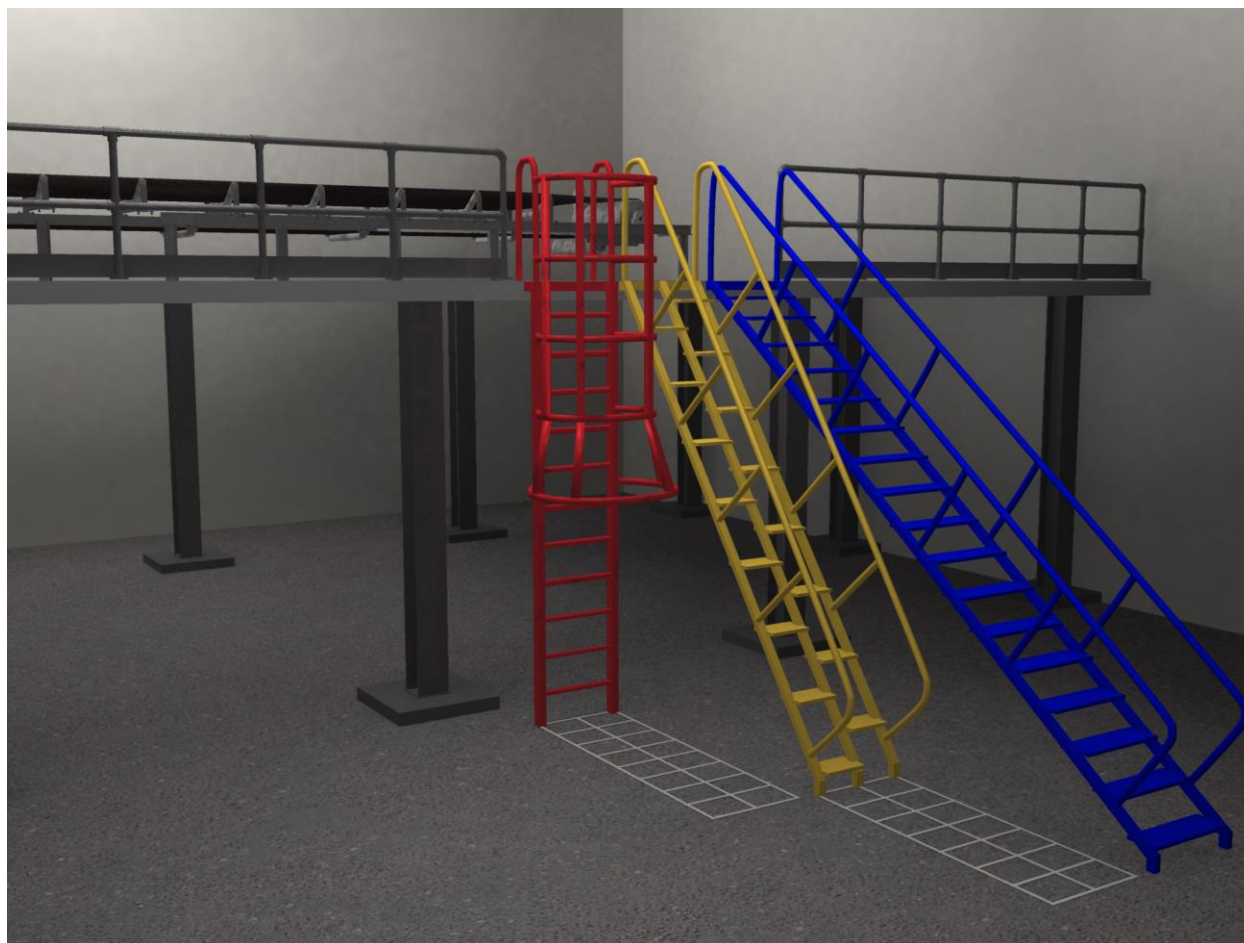
Figure 9.9. Three types of ladder designs. On the left is a vertical ladder, in the center is a ladder with alternating tread stairs, and on the right is a traditional stair design at a mine. The grids on the floor represent the relative footprints of the ladders in comparison to each other. Both the alternating tread and traditional stairs provide ergonomic advantages while also lowering workers' respirable dust exposure compared to a vertical ladder.
