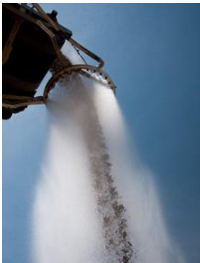
Figure 11.10. A dust suppression ring providing wetting of the product as it is discharged from a conveyor.
