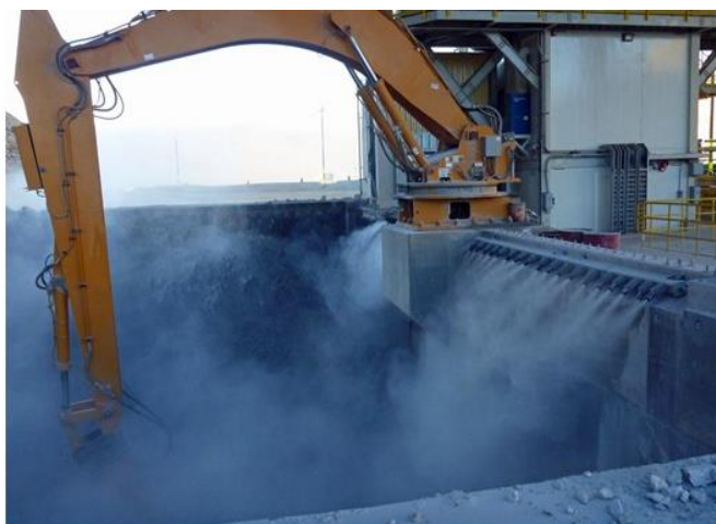
Figure 3.15. Typical dry fog nozzle spray patterns. The left photo shows sprays mounted above a grizzly at a railcar dumper. The right photo shows a primary crusher with nozzle manifolds.
