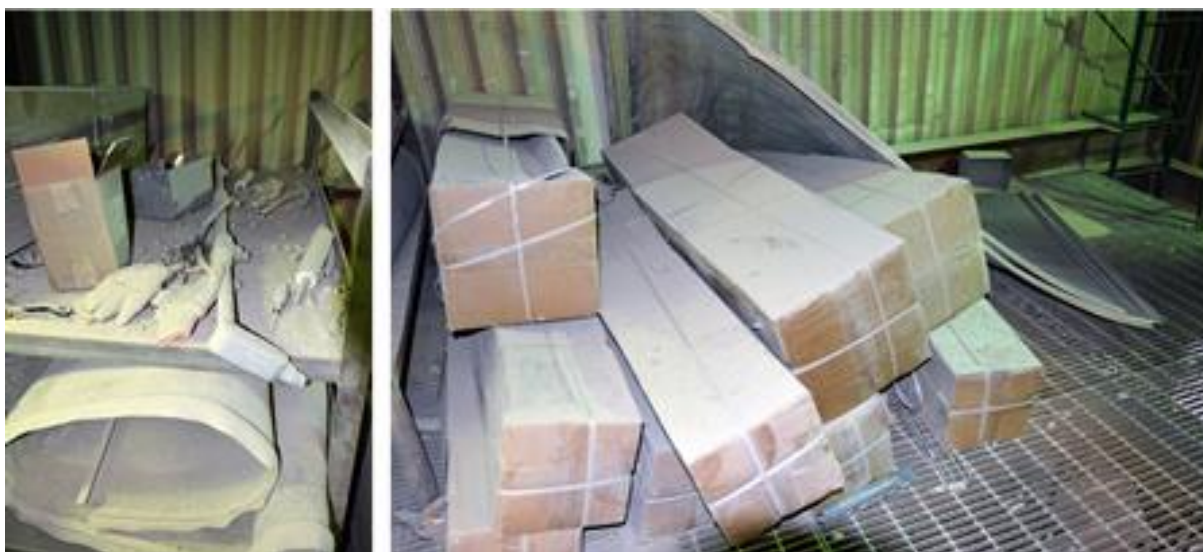
Figure 9.13. Examples of poor housekeeping practices with screens. The left photo shows old screens being stored before disposal. The right photo shows new screens in boxes before use.
