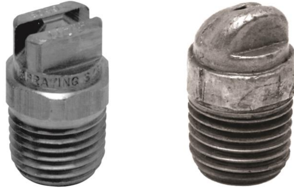
Figure 3.27. Nozzle damage—new versus used [adapted from SSCO 2013].
