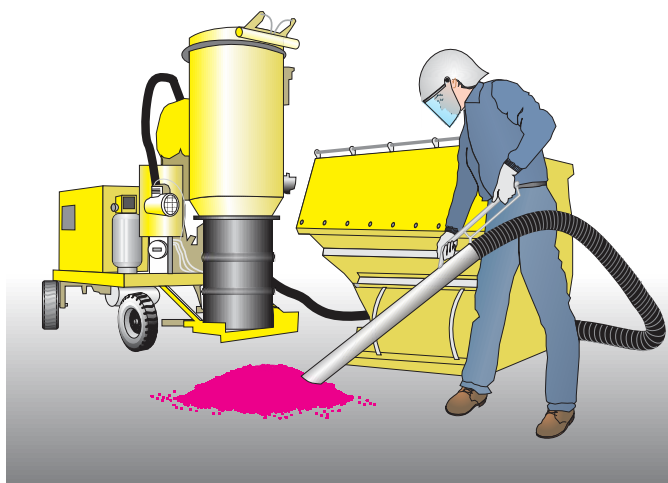
Figure 9.19. Illustration of a portable system used to vacuum product.
