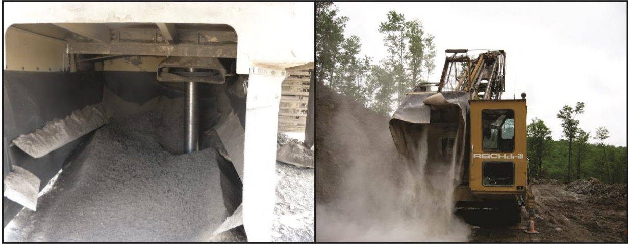
Figure 4.13. Material buildup from drill cuttings that can occur with the use of an air-blocking shelf. The left photo shows buildup of material on the air-blocking shelf. The right photo shows the resulting dust emissions created during lowering of the drill mast.
