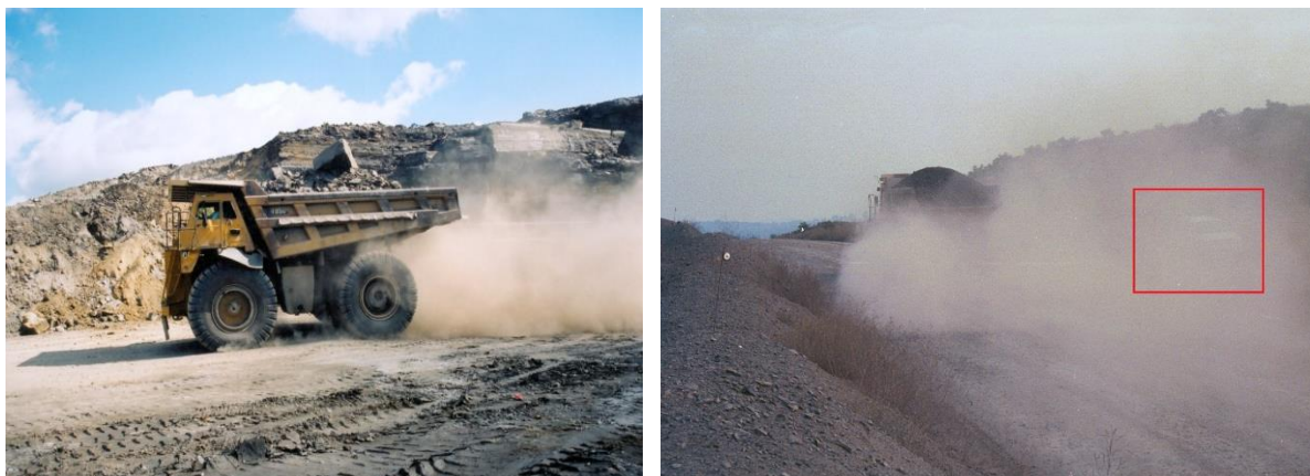
Figure 11.1. Examples of haul road dust from mine haul trucks. The photo on the right, with the red box outlining a light fleet vehicle, shows the level of dust obstruction that can result from dusty haul roads.
