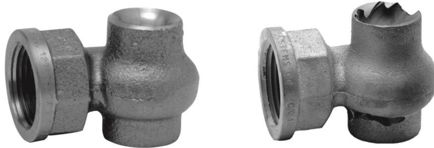
Figure 3.23. Nozzle erosion—new versus used [adapted from SSCO 2013].
