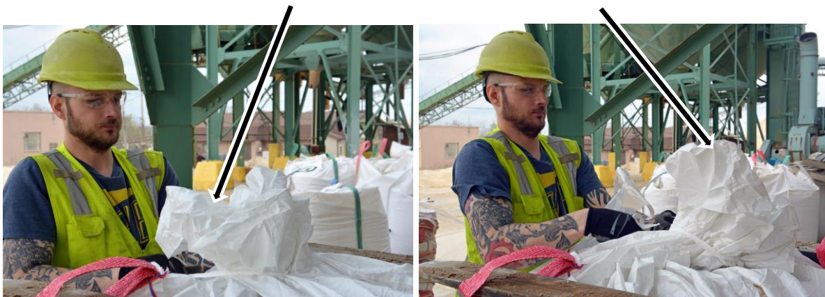
Figure 9.24. Photos representing how a worker's method for tying a bag collar on a flexible intermediate bulk container can significantly impact respirable dust exposure.
