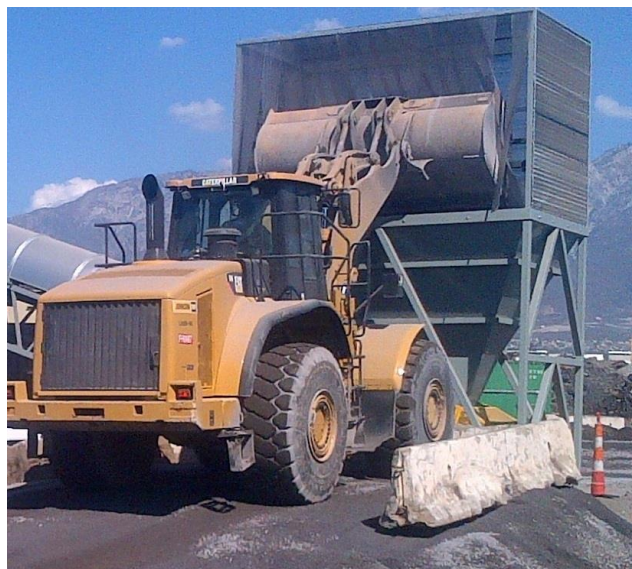
Figure 3.14. Typical wind fence installations. The left photo shows a porous windbreak material around a stockpile drop. The right photo shows the material being used at the top of a loadout hopper.
