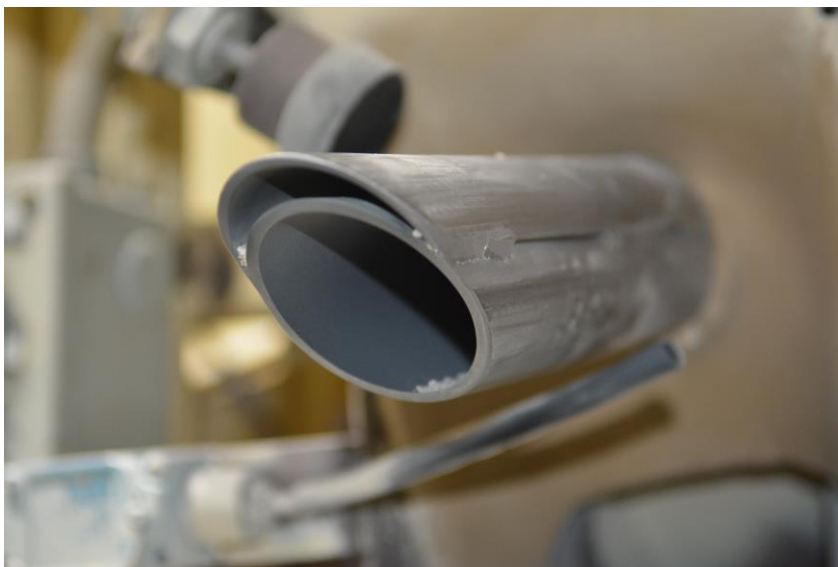
Figure 7.10. Major components of a dual-nozzle bagging system. The top illustration shows an overall design diagram. The bottom photo shows a close-up of a dual-nozzle device.
