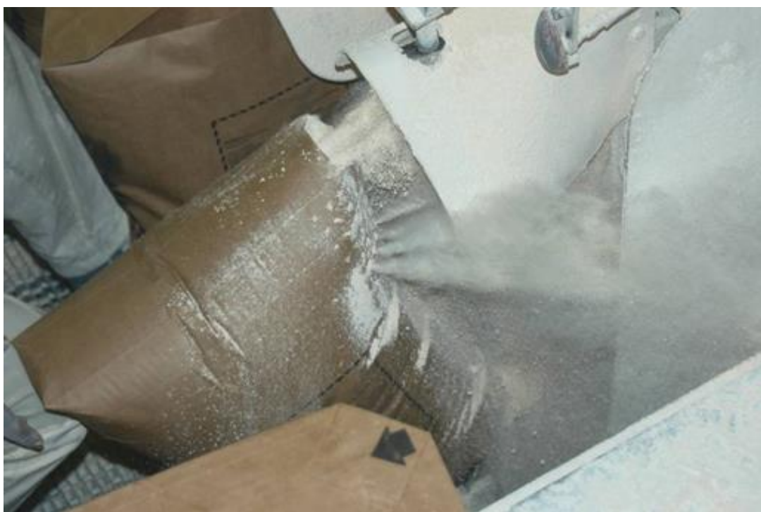
Figure 7.4. Photo showing how undervalue perforations relieve excess pressure from a bag during the filling process to minimize the possibility of bag failure. Product and dust are seen escaping along with excess air.
