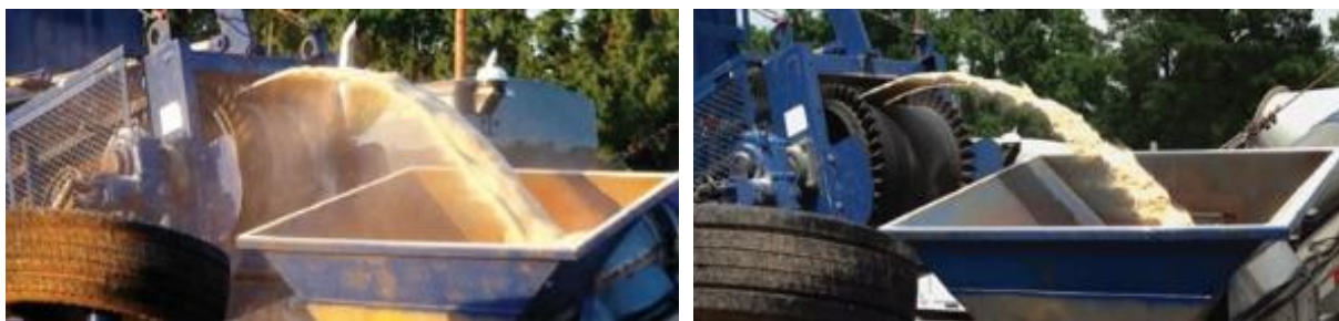
Figure 1.8. Untreated and treated sand being loaded off a conveyor. The left photo shows untreated sand; the right photo shows sand treated with a silica dust control coating technology to reduce silica dust generation.
