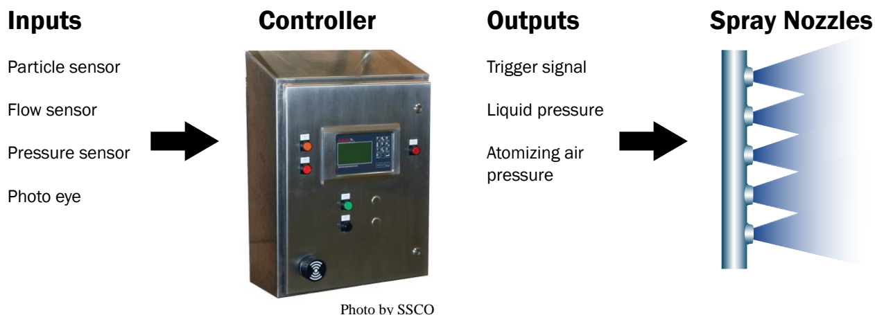
Figure 3.19. Components of a typical automated control system. Arrows indicate flow of the system logic. Inputs feed into the controller and the controller feeds outputs to affect the operation of the nozzles [adapted from SSCO 2018].
