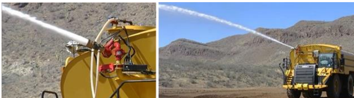
Figure 11.12. Specialized nozzle for wetting large areas. The photo on the left shows a water cannon nozzle mounted on a water truck and the photo on the right shows the nozzle spraying long distances.
