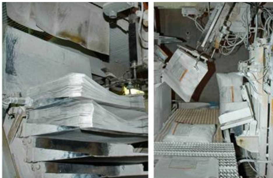
Figure 7.13. Example of a bag storage area and an automated device to place the bag on the fill nozzles. The left photo shows bag storage shelves and the right photo shows a robotic arm with suction cups to place empty bags on the fill nozzle.
