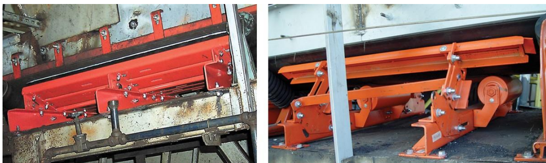
Figure 6.4. Impact cradle and side support cradle. The impact cradle (left) reduces material rebound and spillage, while the side support cradle (right) is specified in “no impact” zones or for lighter-duty ore transfer applications. These cradles are often combined in systems to provide the foundation necessary for properly sealing the belt.
