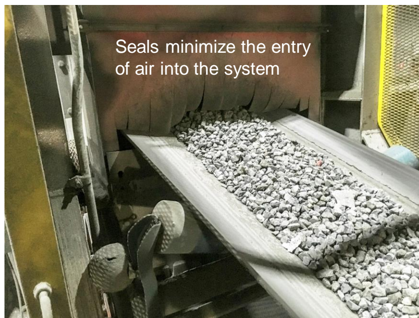
Figure 6.14. Demonstration of material being transported into a sealed head chute.
