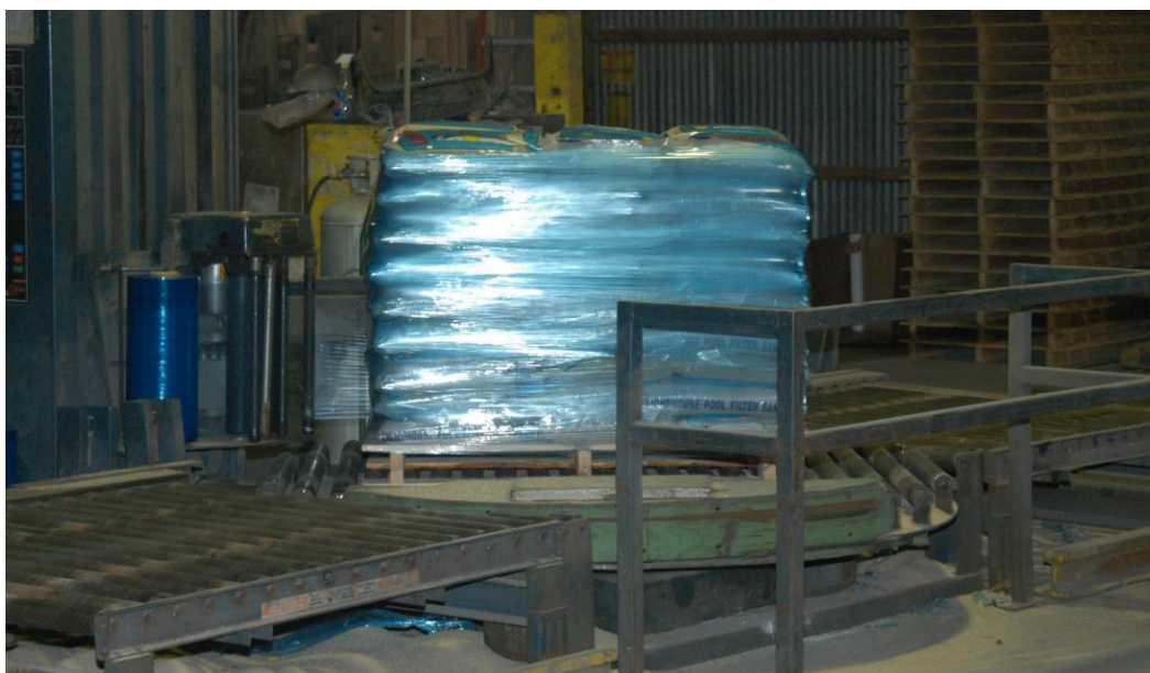
Figure 7.21. Illustration and photo of a plastic pallet wrapping system. The top illustration shows an automated spiral stretch wrap machine. The bottom photo shows the wrapped product on a rotating table.
