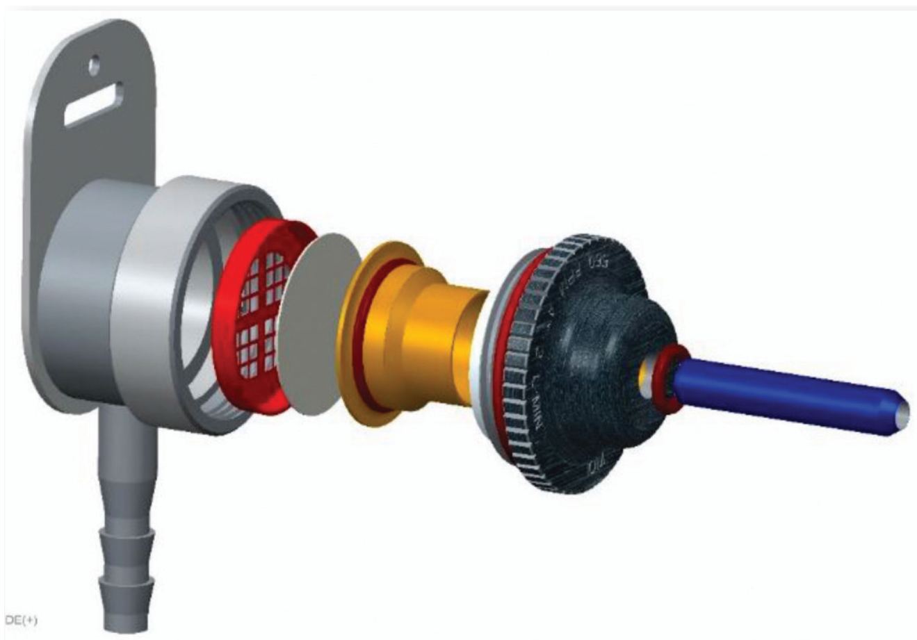
Figure 4. Exploded detail of the total dust sampler, consisting of a commercially available stainless steel IOM sampler with a custom-printed inlet adapter (black) allowing inlet nozzles (blue) of different sizes to be used.
