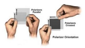
If, however, the light beam strikes an RCS particle with the birefringence property, the polarisation of the light will be changed marginally, thus allowing a small portion of the light through the second polariser. This signal is then picked up by the birefringence detector (see section 1.5). The diagram below further illustrates the technique.
