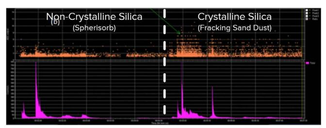
As can be seen in the graphs, both the birefringence signal and the scatter ratio show an identifiable difference between non-Crystalline Silica and Crystalline Silica. By statistically analysing both signals in combination with size data it is possible to identify Crystalline Silica from non-Crystalline Silica.
