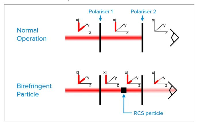
As can be seen in the lower diagram, the beam strikes an RCS particle and changes the polarisation of the light, re-introducing a small horizontal component. As the second polariser is oriented to block the vertical element, this horizontal component passes through and is picked up by the detector. Birefringence can also vary dependent on particle size, so it is essential to combine this data with the size data.
