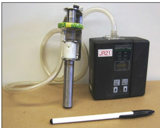
Figure 2-1.—Gravimetric sampling pump, cyclone, and filter cassette.
