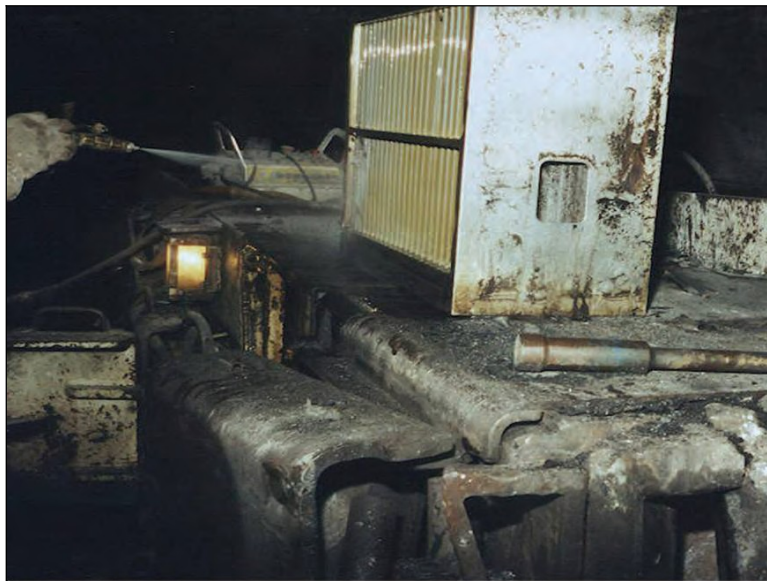
Figure 4-8.—Cleaning the demister with a water nozzle.
