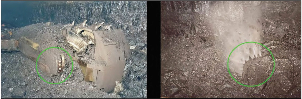
Figure 3-13.—Crescent sprays located on shearer ranging arm.
