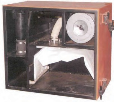
Figure 4-14.—Dust collector box with collector bag installed.
