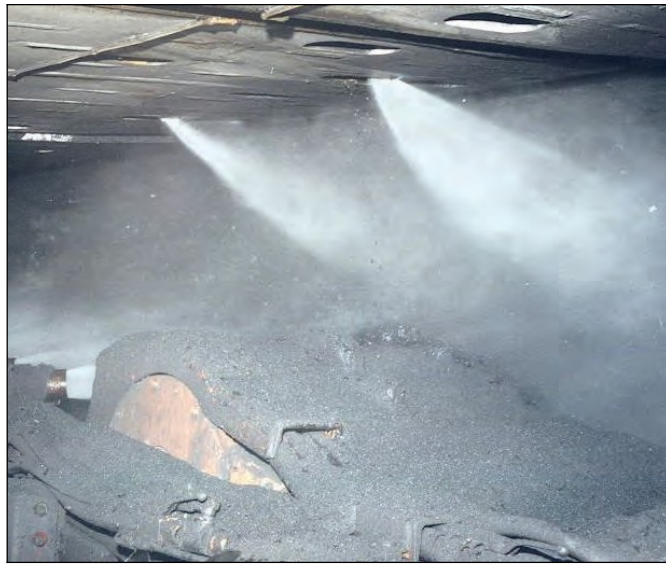
Figure 3-15.—Shield sprays located on the underside of the canopy.
