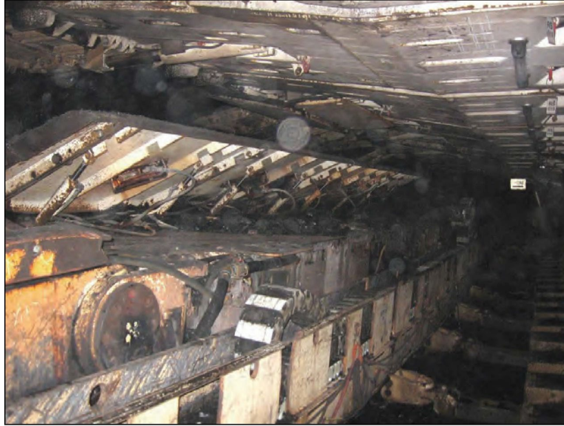
Figure 3-12.—Raised deflector plate can enhance the effectiveness of the directional spray system.
