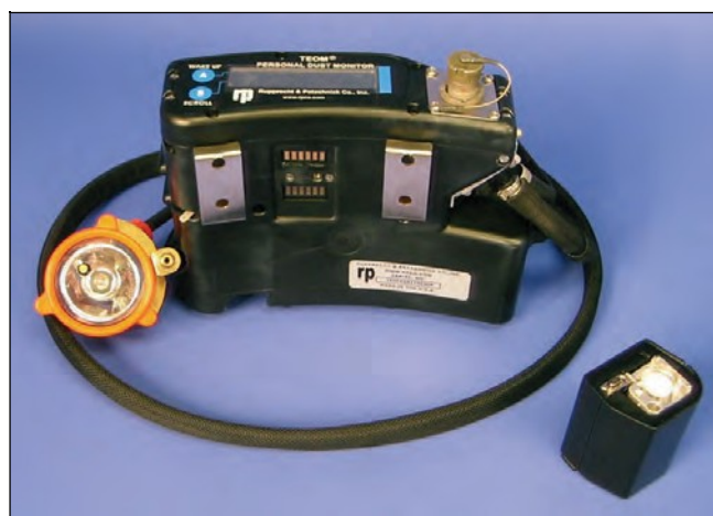
Figure 2-3.—PDM with TEOM removed (shown on right).
