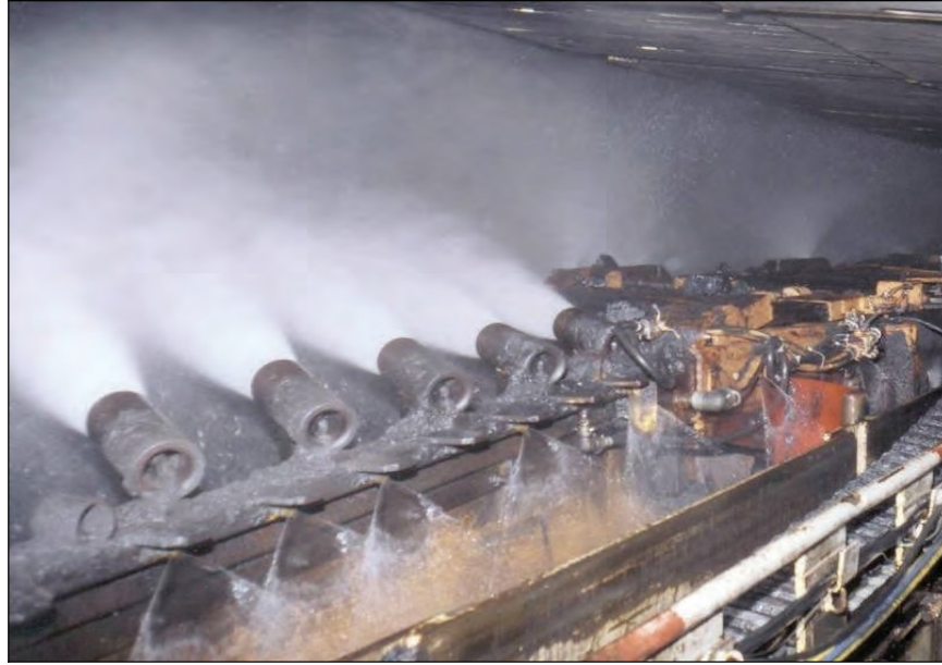
Figure 3-8.—Venturi sprays mounted on headgate splitter arm.
