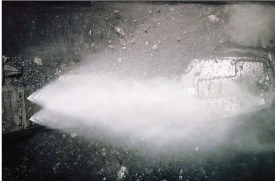
Figure 3-14.—Spray manifold mounted on tailgate end of shearer body.
