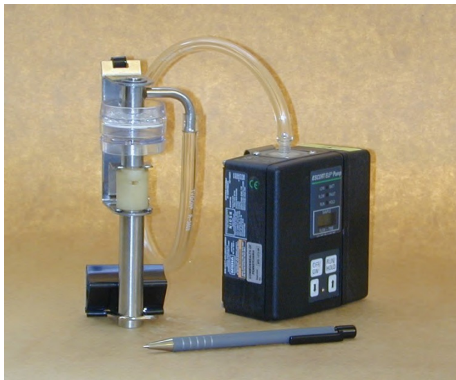
Figure 2-1. Gravimetric sampling pump, cyclone and filter cassette.
