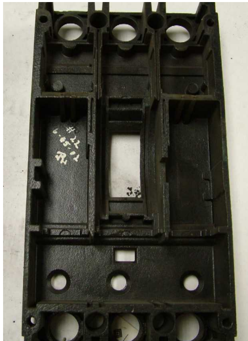
Figure 3: Shot Blasted and Painted
