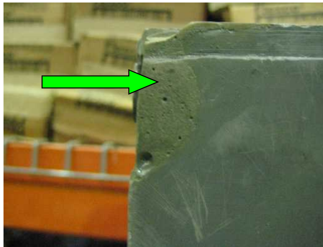
Figure 4: Epoxy Repair to Case Corner
