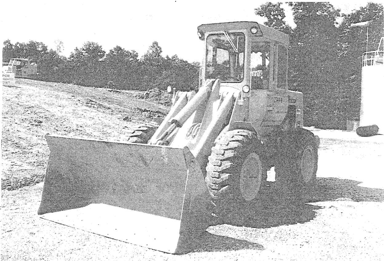
This module describes the basic job steps, potential hazards or accidents, and recommended safe job procedures for front-end loader operation.
