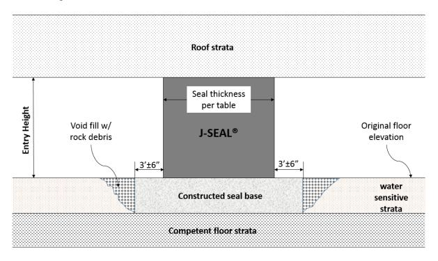
While constructing the base, the excavated cavity can be filled entirely with high strength grout, or similar material. Normal formwork can also be used for construction of the base. The formwork can remain in place or be removed once the base has achieved the minimum UCS per the sampling procedure. The excavated area can be backfilled with dirt and/or rock debris to the approximate original floor horizon.
