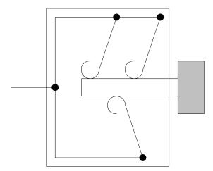
Note: When the connector is completely disconnected, the circuits should remain intrinsically safe.
